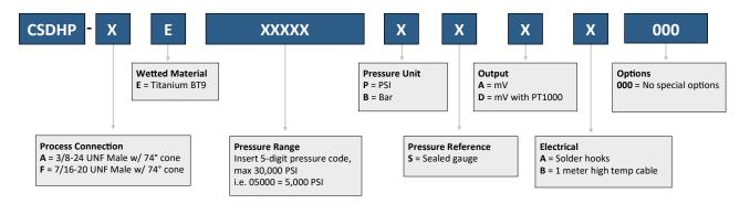
Ordering Example: CSDHP-AE20000PSAA000 (3/8-24 UNF Male w/ 74° cone, Titanium BT9, 0-20000 PSI sealed gauge, mV, Solder hooks) Not all configurations are available. Our sales team can recommend the closest available configuration based on your requirements. Contact Core Sensors for configurations not shown.
