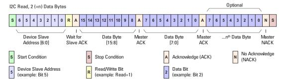
A read command will return the data from the output register. It will not interrupt the normal processing of the ASIC. Three bytes of data should be read... the first byte is the original command (0x2E), the next two bytes are the pressure output in counts.
