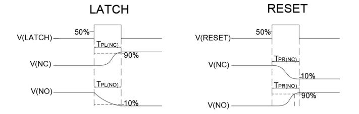
Switching Characteristics (Note: All Signals Measured with Respect to XV Bus Return)
